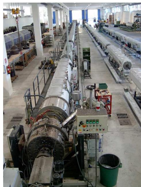
The pipe extrusion die supports and distributes the homogeneous polymer melt around a solid mandrel, which forms it into an annular shape for solid wall pipe.
