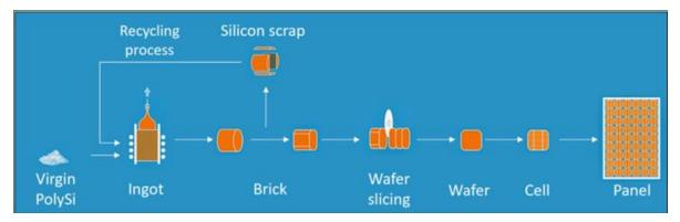
Step 1 - **PolySi**: The raw material used to produce the cells is a high purity silicon called "Solar grade silicon" or "PolySi".
