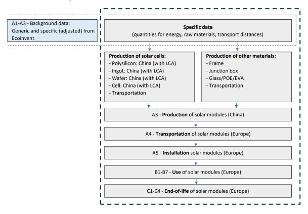
The PolySi, ingots, wafers, cells and modules are manufactured in China. The supply chain is shown below:
