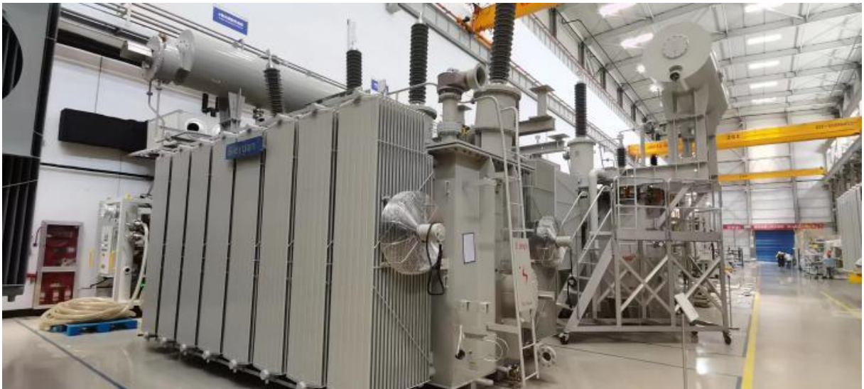
Figure 2.1 - SFZ-40000/115 Oil-immersed power transformer
